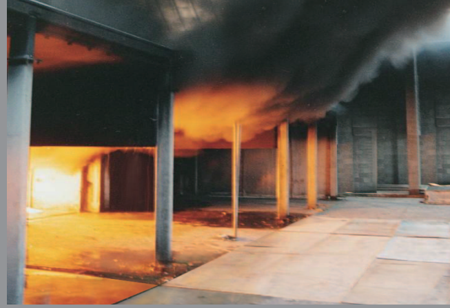
Smoke barrier used in fire testing
